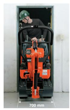
When adjusted down to 700 mm, the K008-3 can easily fit through most doorways, permitting access inside of buildings.
