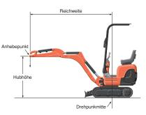
Please note: \* The lifting capacities are based on ISO 10567 and do not exceed 75% of the static tilt load of the machine or 87% of the hydraulic
