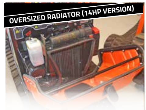
The air/water cooling system allows the machine to operate in extreme conditions
